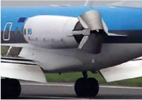
*Typical Thrust Reverser in deployed mode*
