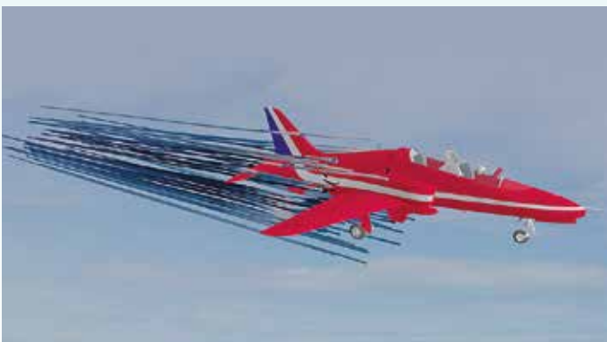
Figure 4 Rendering of relative air velocity over an aircraft approaching landing
